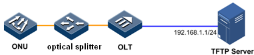
Figure 1-8 Intelligent upgrading ONU
